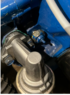
Stock Oil PSI switch shown on 302.
