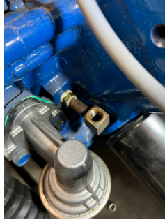
1/4" NPT extension pipe with 90 degree fitting installed.
